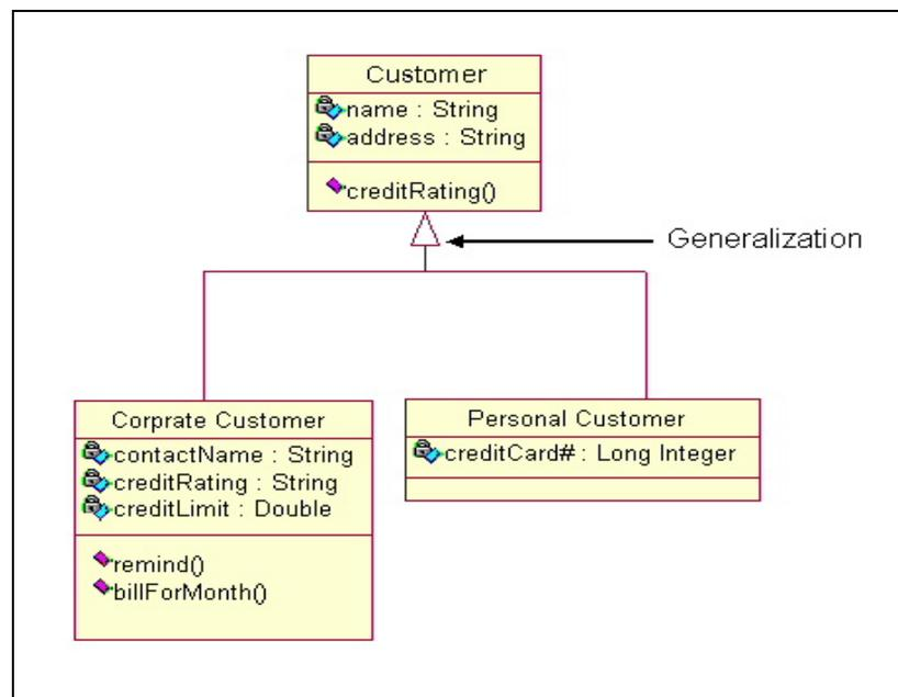
Figure 2.8 Class Diagram Example <sup>[8]</sup>
